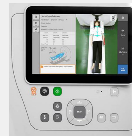
Gantry panel for auto positioning of the patient
