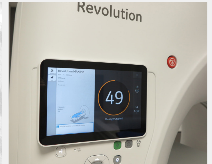
Gantry panel with the option of starting the scan and timing indicator
