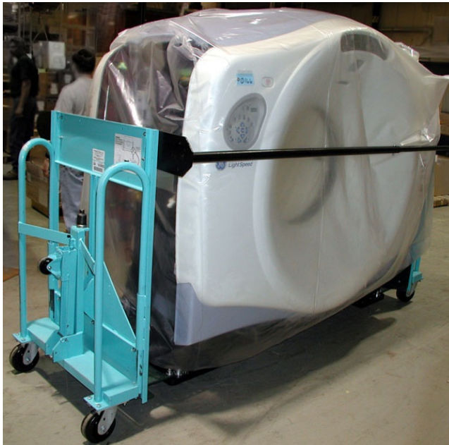
Figure 14-2 Gantry with Heavy Dollies (example)
