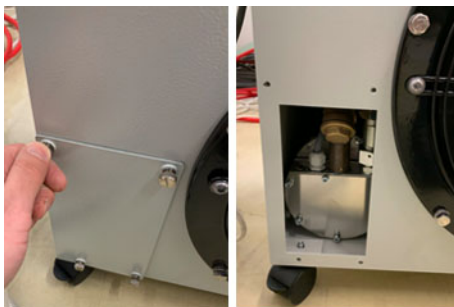
[1]: Cover to access filter strainer
