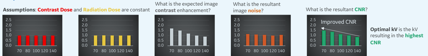
Figure 13. Example demonstrating the three main benefits of Low kV Imaging and their respective assumptions. GE Reference Profiles are designed to provide optimal image quality while reducing radiation dose at lower kVs. Custom User Profiles defined with NI in the profile can be designed in such a way as to reduce contrast dose or increase CNR as kV is reduced. In all scenarios, the optimal kV is dependent on the patient size and clinical task.
