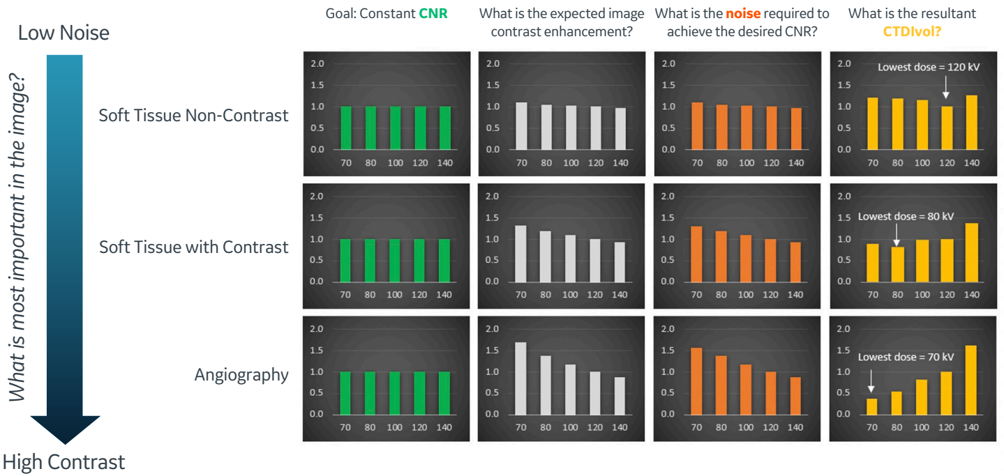
Figure 14. The impact of clinical task on optimal kV for a given patient size, where optimal kV is the kV resulting in the lowest CTDIvol for a desired image quality, defined by CNR.
