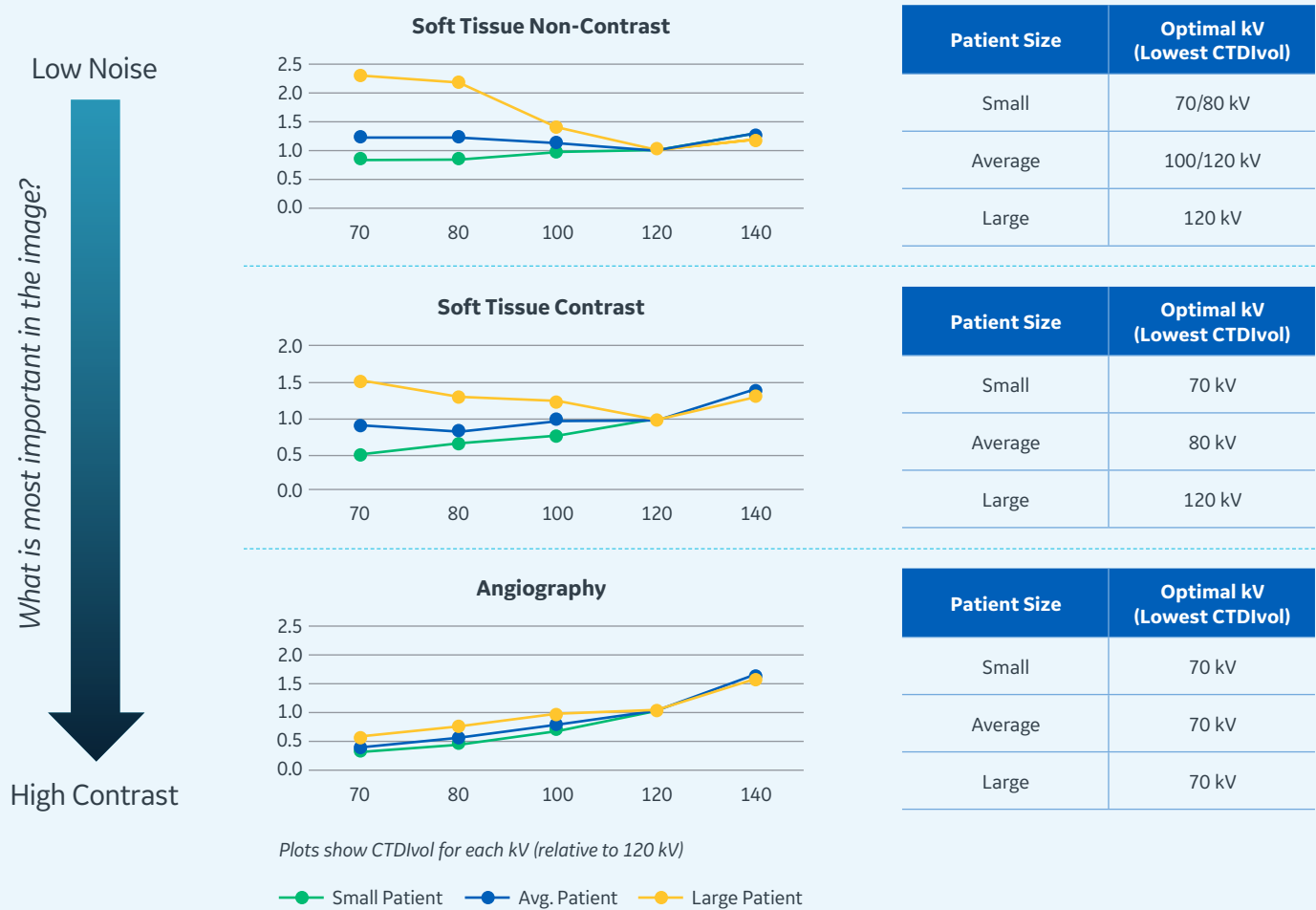
Figure 16. Optimal kV is dependent both on clinical task and patient size. In this figure, the optimal kV for each patient size is the one with the lowest CTDIvol. Note that this figure does not consider tube power limitations. The actual optimal kV will also depend on which kV can achieve the Prescribed Noise Index.
