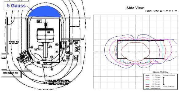
Typical Shielding: 5 Gauss Line Containment Back Wall
