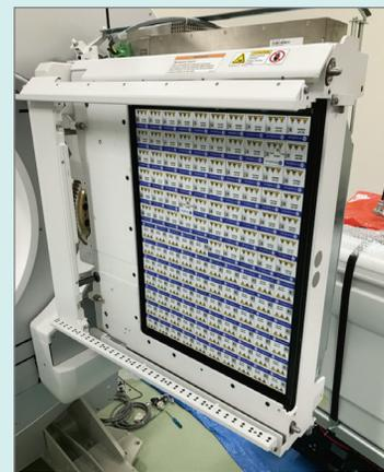
**Figure 1.** The CZT detector without collimator. CZT detector modules are aligned to the edge of the frame and the brain reach is 2.5 cm.
