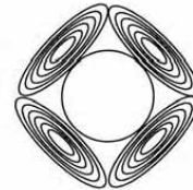
Oscillating bubble and microstreaming
