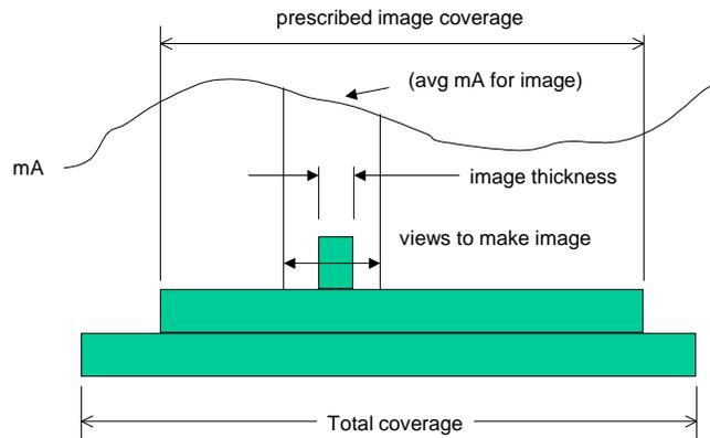
$$\text{exposure} = (\text{exposure time}) * (\text{image avg mA}) * (\text{slice thickness}) / (\text{total coverage})$$
