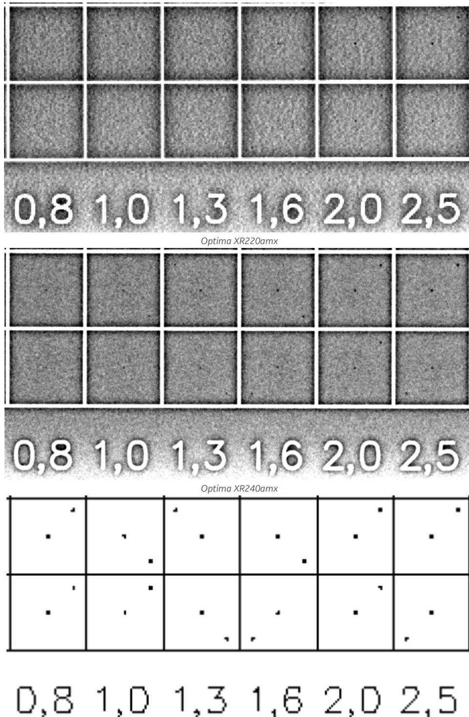
**Fig. 12:** Example of CDRAD image for condition 1 with 4mAs, holes diameter is 0.4mm on the top line and 0.3mm on the bottom line
