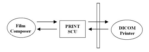
The Film Composer is the User interface and this is used to initiate the local real world activity. The user issues the print request using Film Composer. Film composer allows printer selection and it composes the pre-formatted film file. This film file is interpreted by Print SCU and it sends the appropriate messages to DICOM print SCP running on a DICOM printer.
