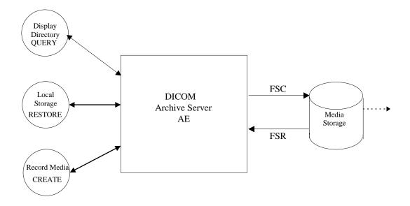
The DICOM Interchange Archive Server AE has a local storage that may contain various SOP instances. These may have been obtained by original creation, network (DICOM or proprietary) or by removable media using other application entities. These instances are external to this conformance claim and the origin of SOP instances is outside the scope of this claim.
