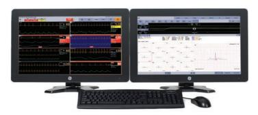
A secondary display extends the work surface of the primary central station and is dedicated to the review of a single patient's data. One keyboard and mouse can be shared across the primary central station and the secondary display.
