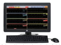
A mirror display provides an interactive workstation, displaying the same patients as the primary central station. Changes made at the primary central station are reflected at the mirror display and changes made at the mirror are reflected at the primary.
