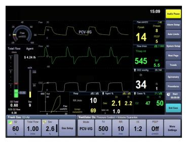
**Figure 2.** ecoFLOW display on the Aisys  $CS^2$  anesthesia machine showing fresh gas flow settings in the bottom left panel. The  $FiO_2$  indicator can be seen on the Total Flow tube (green) and the Agent cost can be seen in the ml/h tube indicator (yellow).
