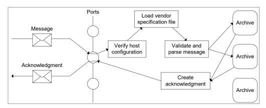
It is also assumed that a connection is closed when it is idle. For example a connection may be set up for the sending of one message and one acknowledgment and can be closed. The current implementation closes a connection if it has been idle for more than 300 seconds, resulting in a time-out message in the log. There is no upper limit to the number of simultaneous connections that can be opened.
