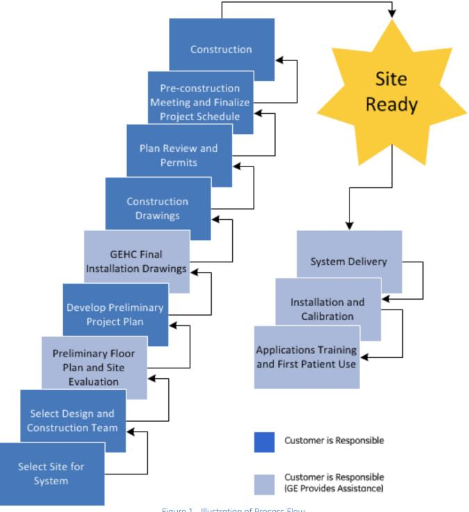
Figure 1 - Illustration of Process Flow
