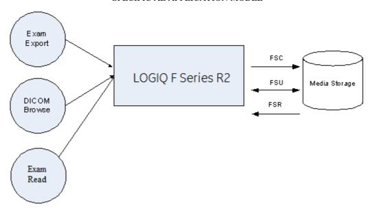
LOGIQ F Series R2 can initialize Media by acting as an FSC to create a new DICOM File-set on CD/DVD media of various sizes. The SOP instances written to media must be one of the instances supported by LOGIQ F Series R2. A pre-existing File-set will be updated with the information in DICOM files copied to media.
