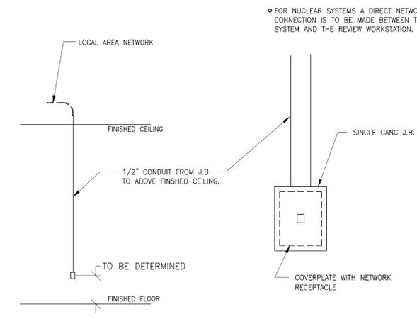
FOR NUCLEAR SYSTEMS A DIRECT NETWORK CONNECTION IS TO BE MADE BETWEEN THE SYSTEM AND THE REVIEW WORKSTATION.
