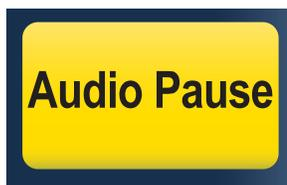
Selecting **Audio Pause** for an active alarm stops the audible tone for 120 seconds. The alarm message shows in the alarm message field. Selecting **Audio Pause** when no medium or high priority alarms are active prevents the audible alarm tones (audio off) for 90 seconds.
