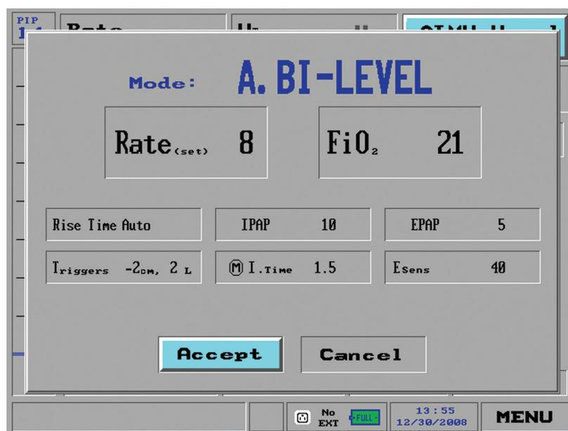
Figure 4.7 Adaptive Bi-level parameter window
