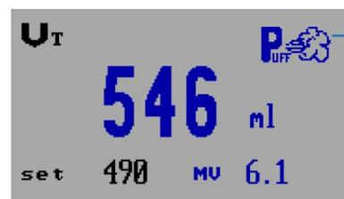
**Blue P:** Purge sensor lines function is activated. To help prevent moisture build up when a humidifier is connected, the iVent<sub>201</sub> will send a puff of high pressure air through the sensor lines to clean them.
