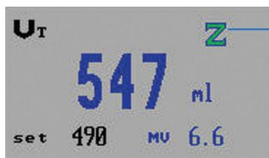
**Green Z:** Automatic Zeroing of Sensors: The iVent<sub>201</sub> has calibrated itself to ensure that the sensors are measuring accurately.
