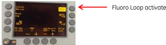
3. When fluoro is started, fluoro images begin to store. When fluoro is stopped, the acquired loop will automatically begin playback. (Configurable)
