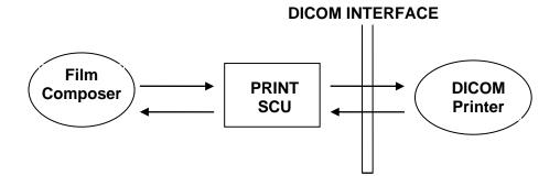
The Film Composer is the User interface and this is used to initiate the local real world activity. The user issues the print request using Film Composer. Film composer allows printer selection and it composes the pre-formatted film file. This film file is interpreted by Print SCU and it sends the appropriate messages to DICOM print SCP running on a DICOM printer.
