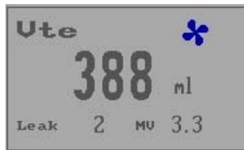
Figure 129: Leak Estimated Value in LPM
