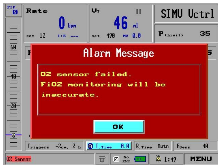
Figure 85: Low+Monitoring O2 Sensor Failed Alarm Message
