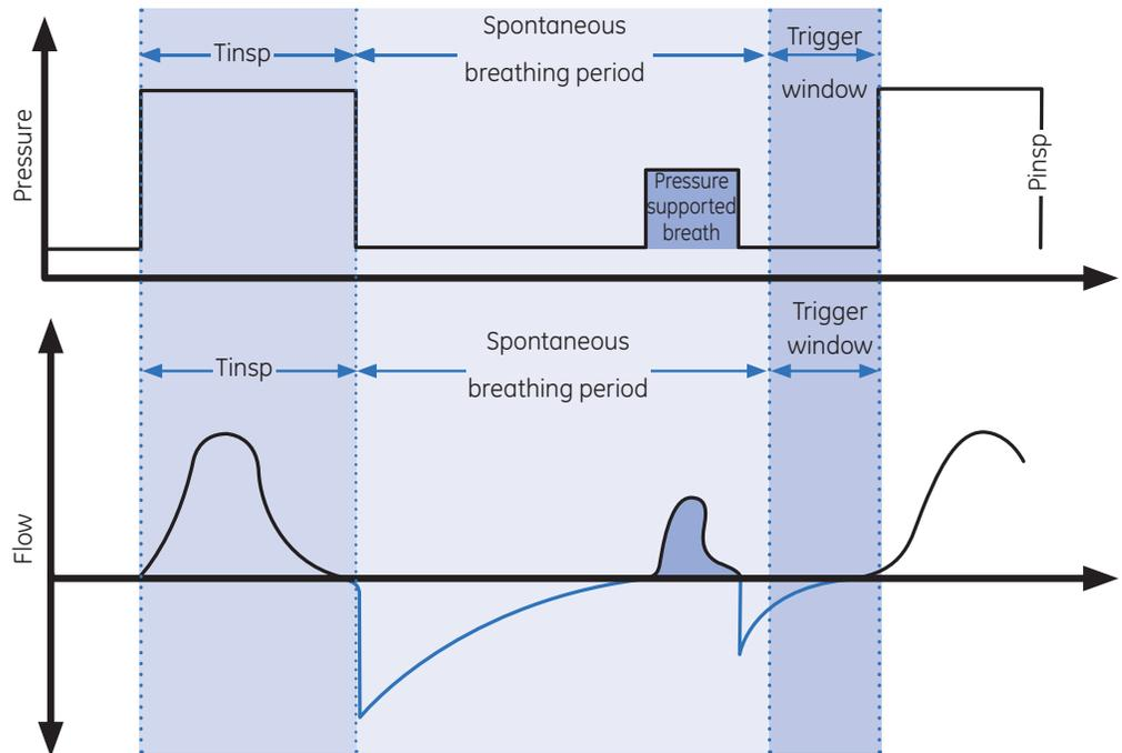
Figure 7.11 Example of Pressure and Flow Waveforms
