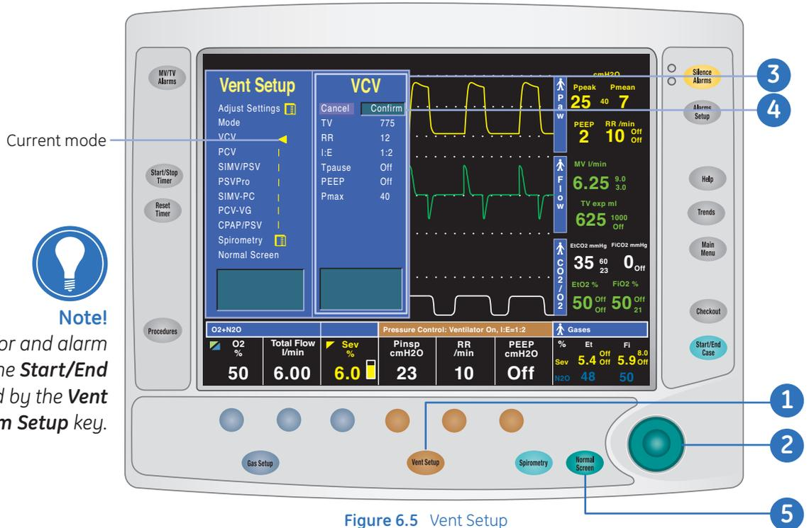
**Adjust Settings:** Adjust settings of the current ventilation mode. Available settings on the secondary menu are specific to the vent mode. Some settings can also be adjusted using the Quick Keys.
