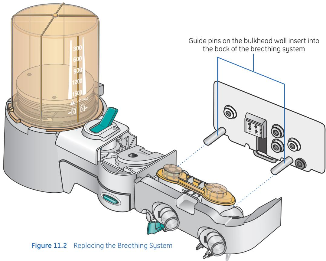
**Figure 11.2** Replacing the Breathing System
