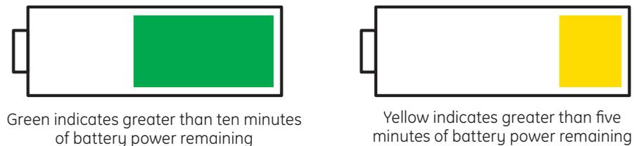
Figure 2.6 Battery Power
