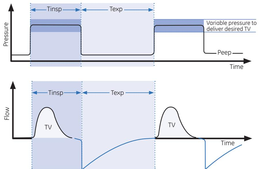
Figure 7.13 Example of PCV-VG Waveforms
