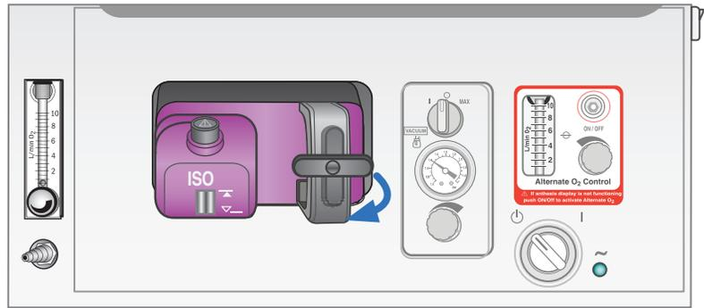
Figure 4.5 Remove the Aladin<sub>2</sub> Cassette
