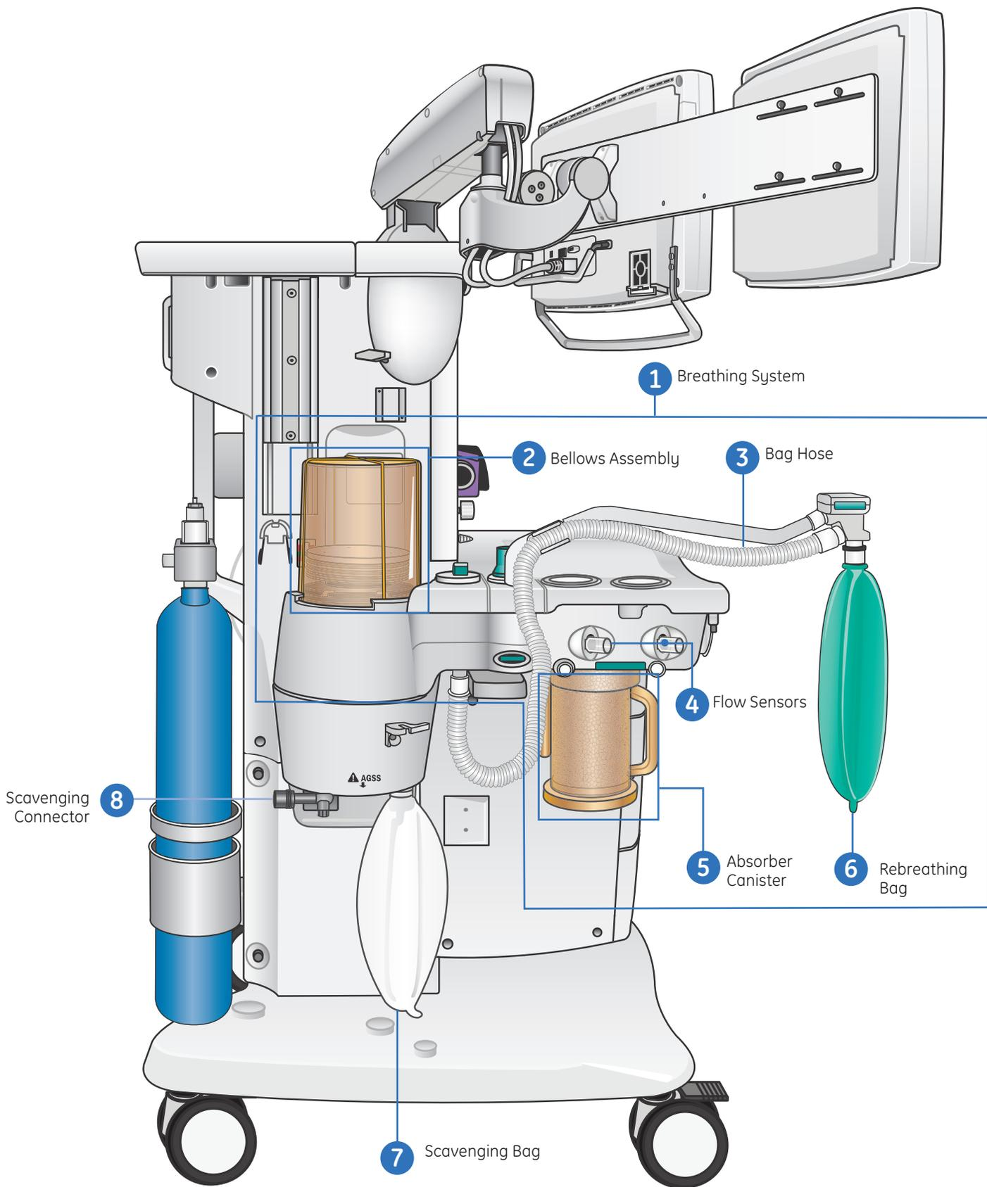
Figure 2.2 Aisys Side View
