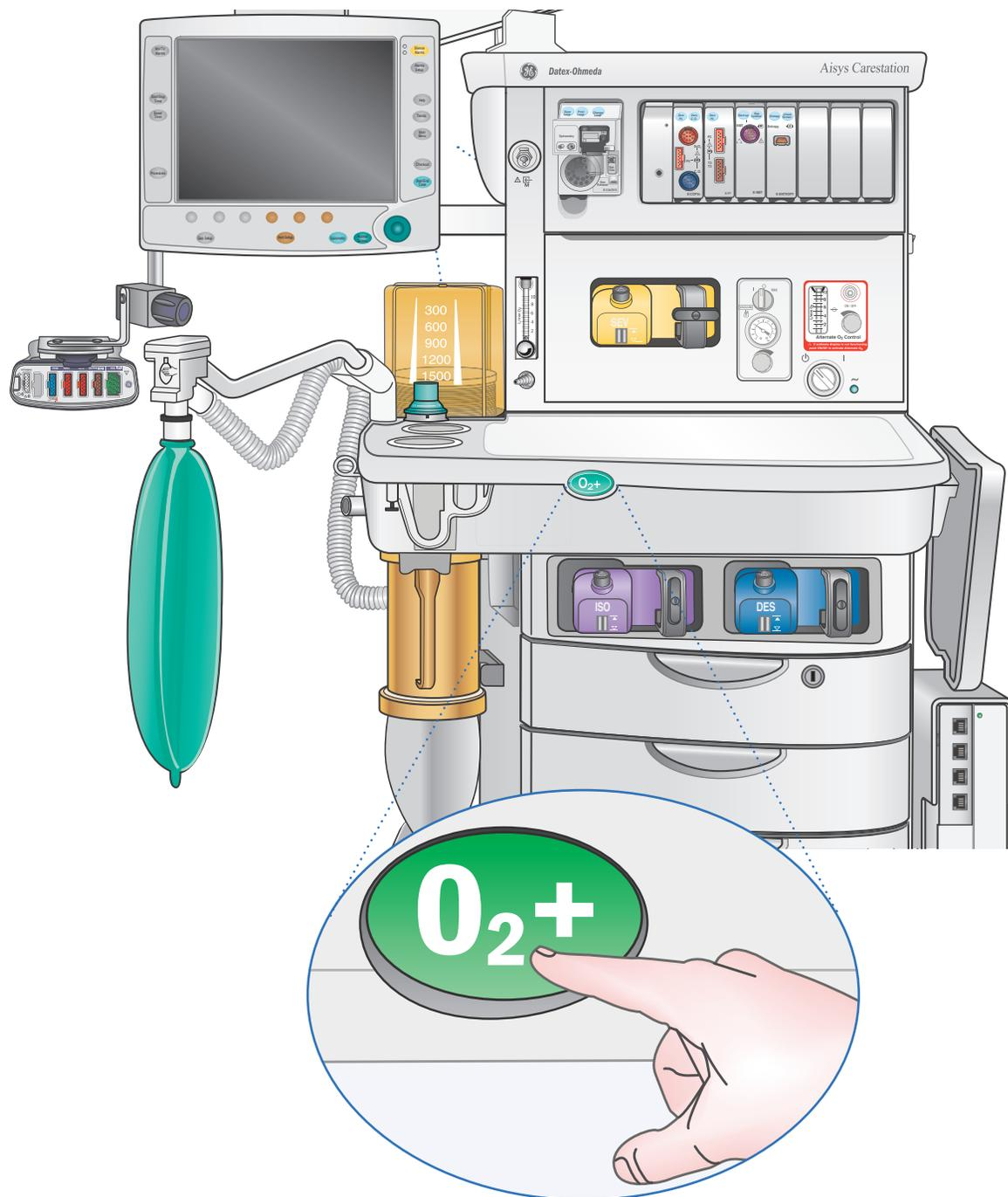
Figure 2.9 O<sub>2</sub> Flush Button
