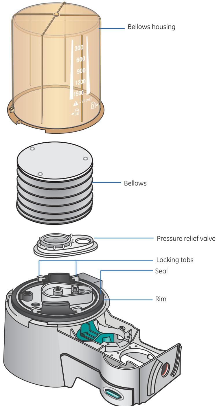
Figure 11.8 Bellows Assembly
