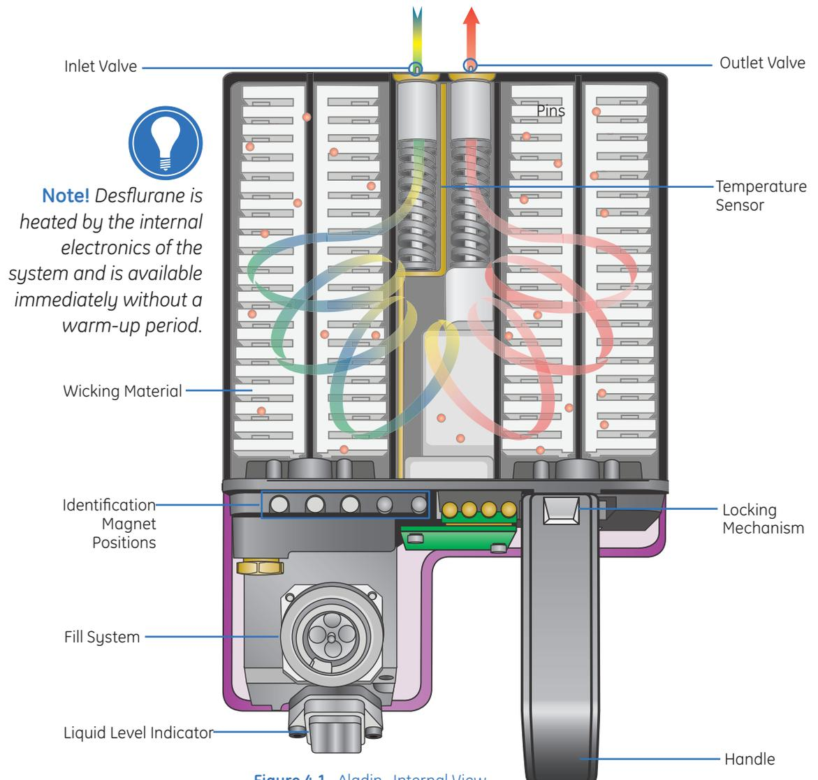
Figure 4.1 Aladin<sub>2</sub> Internal View
