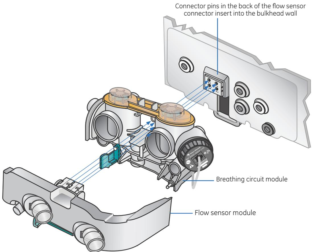
Figure 11.5 Replacing the Flow Sensors
