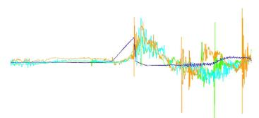
The graph above represents the motion of several parts of the system when it is shaken in a test environment. The blue line is the table motion, the other lines represent motion of the system components.
