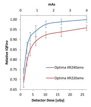
**Fig. 9**: Relative IQFinv of Optima XR240amx and Optima XR220amx systems for condition 1: no additional PMMA filtration, 60kV, SID 120cm
