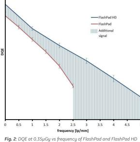
**Fig. 2**: DQE at 0.35μGy vs frequency of FlashPad and FlashPad I detectors
