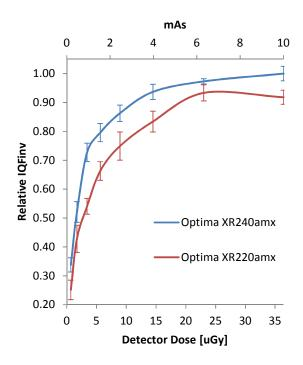
**Fig. 10**: Relative IQFinv of Optima XR240amx and Optima XR220amx systems for condition 2: 10cm additional PMMA filtration, 80kV, SID 120cm
