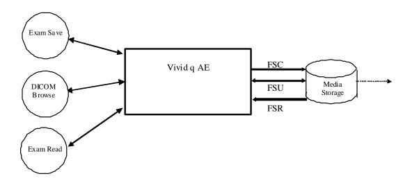
Vivid q can initialize Media by acting as an FSC to create a new DICOM File- set on Media as stated in 3.3.1. The SOP instances written to media must be one of the instances supported by Vivid q. A pre-existing File-set will be updated with the information in DICOM files copied to media.
