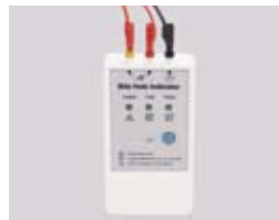
Leak Path Indicator Tester
