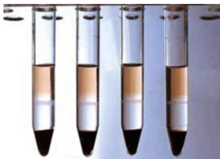
Ficoll-Paque is a density gradient medium that is used for the isolation of human lymphocytes from peripheral blood. Following centrifugation, lymphocytes appear as a distinct white band in Ficoll-Paque.
