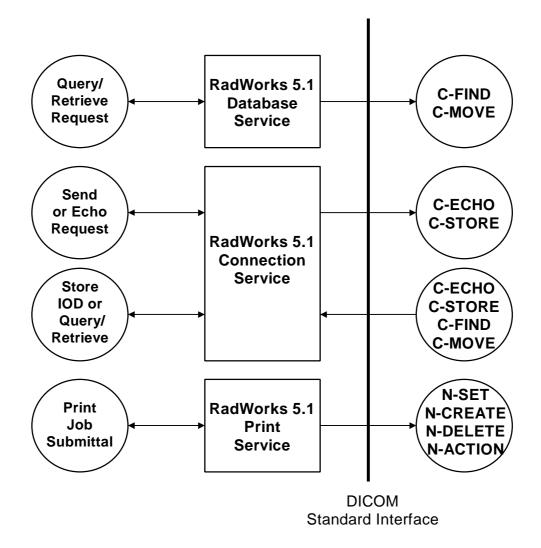
The RadWorks 5.1 DICOM services are implemented as three separate Windows NT Services that run as background processes. They are started automatically during system start-up and will remain active until shutdown. This means that requests for, e.g., image storage can be accepted at all times when the system is up and running regardless of whether the RadWorks 5.1 application is active or not.
