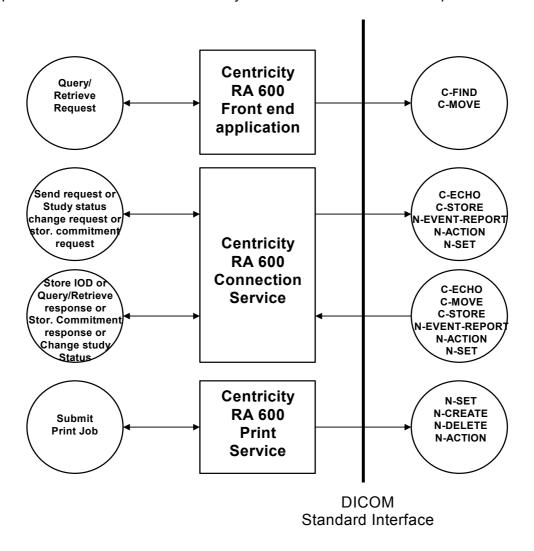
The Centricity RA 600 DICOM services are implemented as three separate Windows services that run as background processes. They are started automatically during system start-up and will remain active until shutdown. This means that requests for, e.g., image storage can be
